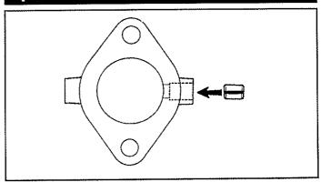
If new bushes are required, we recommend the fitment of the modern teflon-coated steel backed type as supplied in our kits.
